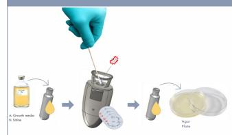
Moistened swab with bacteria suspension applied directly onto nozzle after daily use. Test temperature 32 °C.
